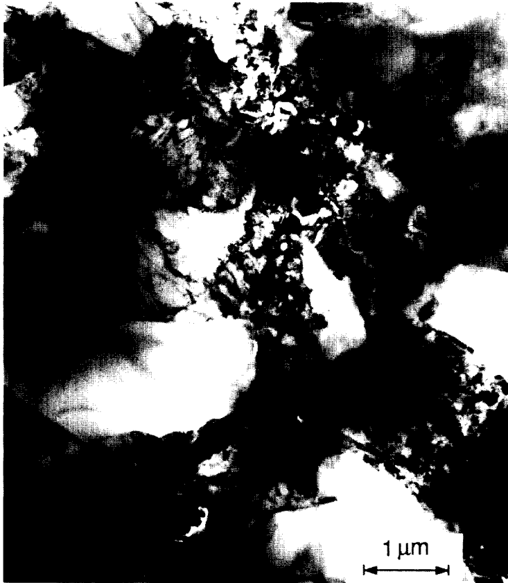
Fig. 1. TEM bright field image showing the AlN filler particles and the AlN/Al matrix.
